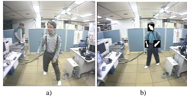
Fig. 6. Visual cues: a) Motion Cue: Detection of a person moving, b) Contextual cue: Human Upper Body Detection
