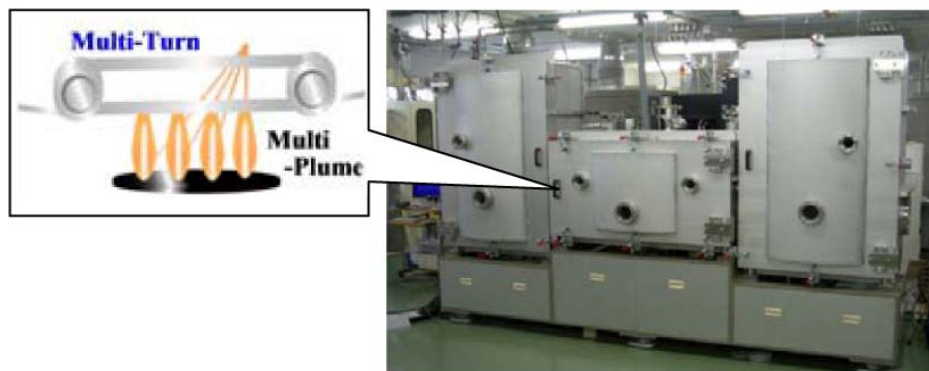
Fig. 12. The PLD fabrication system
