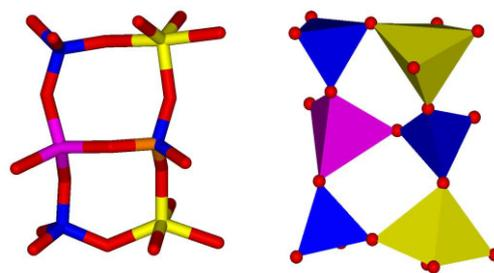
Fig. 1. Stick and polyhedral views of  $\text{Ga}_3\text{P}_3$  hexamer structural units. (blue:  $\text{PO}_4$  tetrahedron, purple:  $\text{GaO}_4$  tetrahedron, yellow:  $\text{GaO}_4\text{F}$  trigonal bipyramid).
