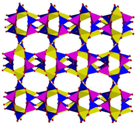
Fig. 4. Polyhedral view of  $\text{Ga}_3\text{P}_3\text{O}_{12}\text{F}\cdot 0.5(\text{C}_8\text{H}_{22}\text{N}_2)$  with 8-ring and 4-ring channels along the [101] direction. (blue:  $\text{PO}_4$  tetrahedron, purple:  $\text{GaO}_4$  tetrahedron, yellow:  $\text{GaO}_4\text{F}$  trigonal bipyramid).
