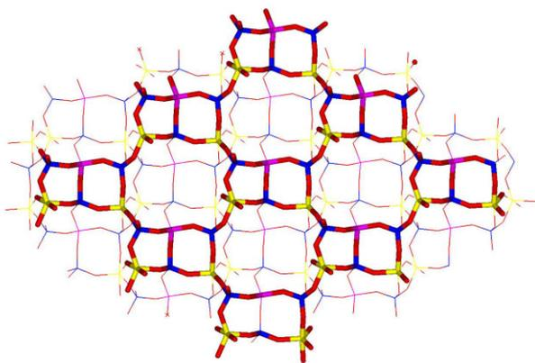
Fig. 3. Stick view of inorganic Layer-D containing 10- and 4-rings along [010] direction. (blue:  $\text{PO}_4$  tetrahedron, purple:  $\text{GaO}_4$  tetrahedron, yellow:  $\text{GaO}_4\text{F}$  trigonal bipyramid).
