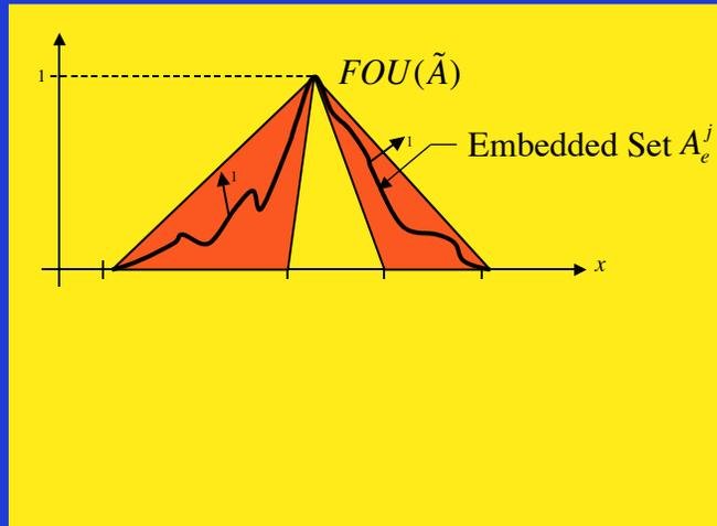
An *embedded set* (also called an *embedded T1 FS*) is a function that lies within or on the FOU.
