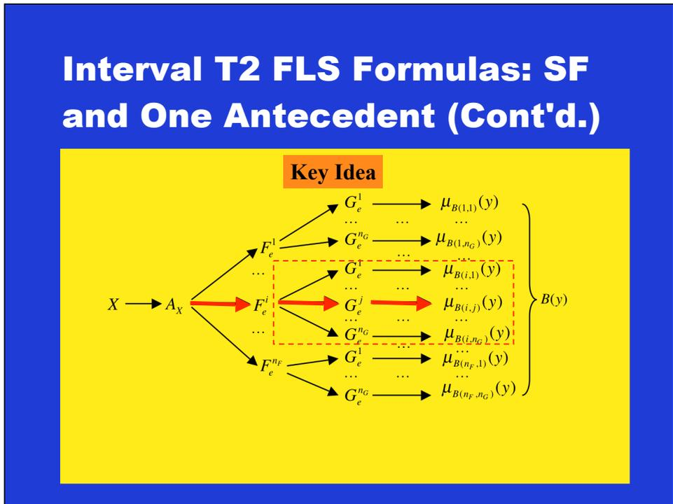
This is a *directed graph* showing (from left-to-right) the singleton input (fuzzified into  $A_x$ ) fanning out into *each* of the  $n_F$  embedded T1 FSs of the antecedent. Each of these then fan out into *each* of the  $n_G$  embedded T1 FSs of the consequent. In total, there are  $n_F \times n_G$  paths. A group of  $n_G$  such paths is enclosed by the red dashed rectangle, and the path shown with red arrows is one such path.
