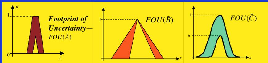
The left-hand FOU was obtained by beginning with a triangle primary MF and assuming uncertainty only about its apex. Assume the uncertainty is given by the interval  $[m - a, m + a]$ . Now beginning at  $m$  slide the triangle  $a$  units to the left and  $a$  units to the right. Doing this you will obtain the filled-in FOU.
