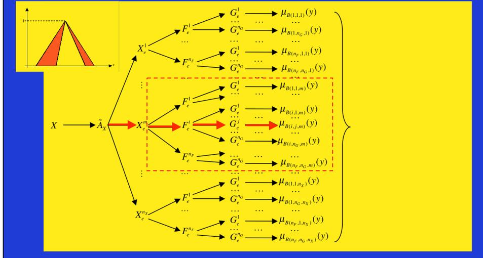
Returning to the case of a single antecedent rule, this time the single input is modeled as an IT2 FS. A representative FOU for the input is shown in the upper left-hand insert.
