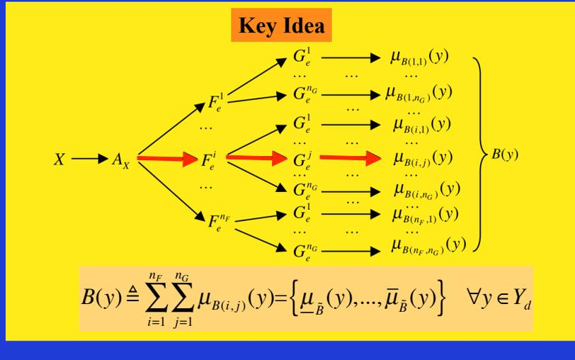
All of the  $n_F \times n_G$  T1 FS s are unioned in order to obtain the MF of the fired rule consequent set of the rule.
