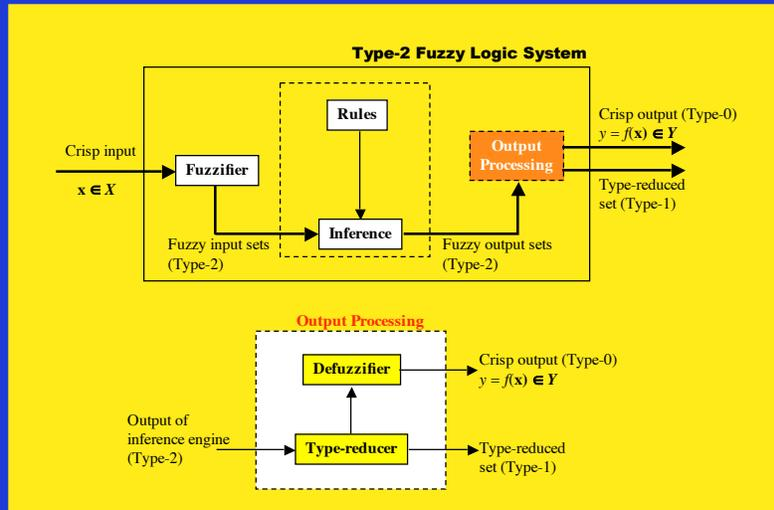
Usually, the desired output of a FLS is a number. *Output Processing* maps the fired rule IT2 FSs into a number, but it does so in two steps.
