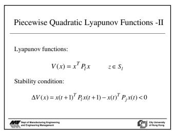
Piecewise Quadratic Lyapunov Functions -II Stability condition:  $A_k^T P_l A_k - P_l < 0 \qquad l \in \overline{L} \qquad k \in K(l)$   $A_k^T P_j A_k - P_l < 0 \qquad (l, j) \in \overline{\Omega} \qquad k \in K(l)$ Interpret of Manufacturing Engineering
