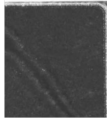
Acoustic microscope image of thermoplastic bonded interface with no defects
