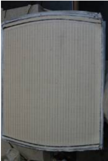
Deployable Exoskeleton Composite w/ Embedded Heating System
