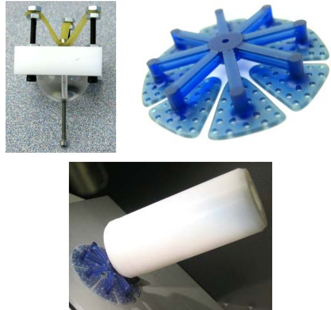
Figure 5: From top left, clockwise: Spherical joint mockup, flexible sticky foot, and prototype foot assembly gripping anodized aluminum.
