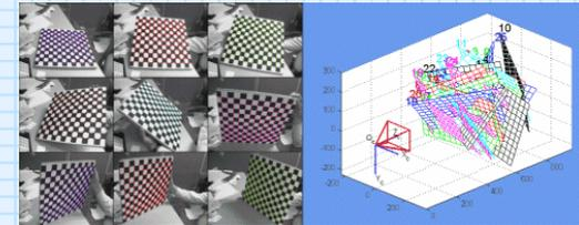
Resulting accuracy in position =  $\sim 1$  mm, in angle =  $\sim 0.1$  deg
