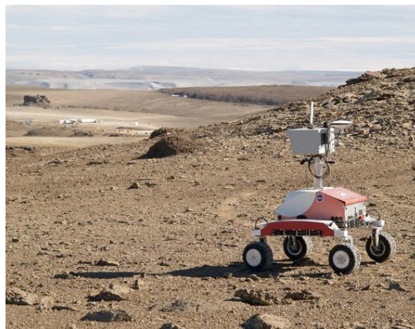
Figure 2. K10 "Red" mapping terrain at Haughton Crater with 3D scanning lidar.
