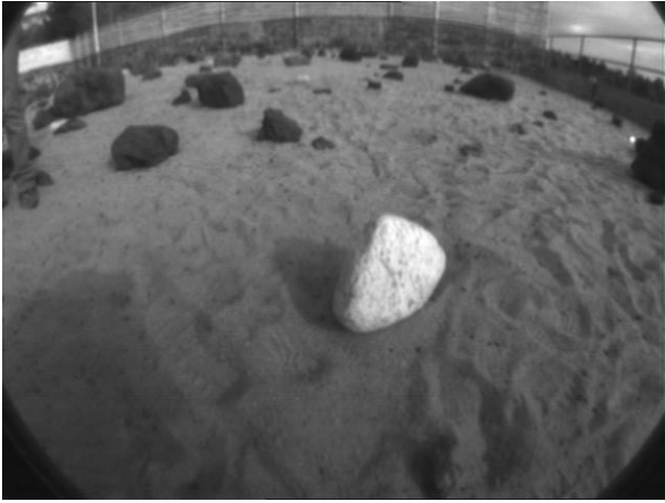
Fig. 2. Image taken in response to a science alert on the JPL FIDO rover. In this test, science alerts were generated for “high albedo” (or light-colored) rocks.
