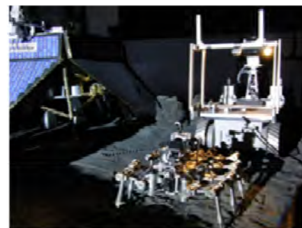
(k) Autonomous docking of Scout and Rover
