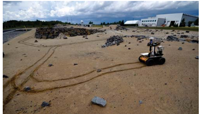
Fig. 1. Rover adding to a network of reusable paths on the Canadian Space Agency’s Mars Emulation Terrain; once created, it can return accurately to any previously visited place using only visual feedback.
