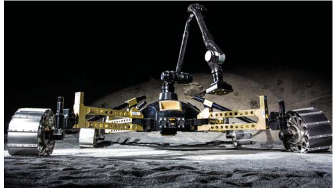
Fig. 1. The planetary rover Sherpa in a flat stance configuration of its active locomotion platform.
