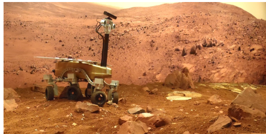
Fig. 1. Planetary rover “Mawson” used for experimental validations, shown in the Mars yard at the Powerhouse Museum in Sydney, Australia.
