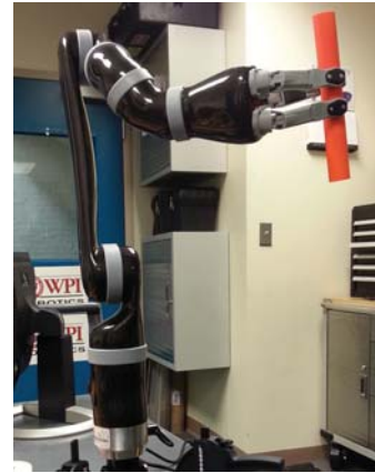
Fig. 3. Jaco 6-DOF manipulator with one of the easy samples grasped.
