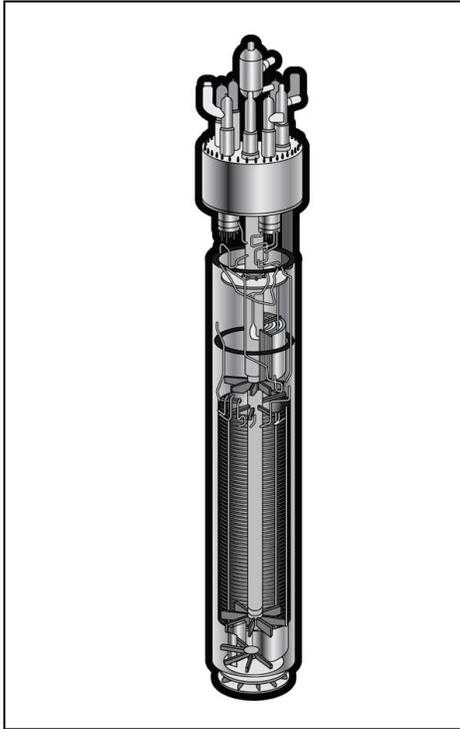
Fig. 1. Diagram of a pod boiler.
