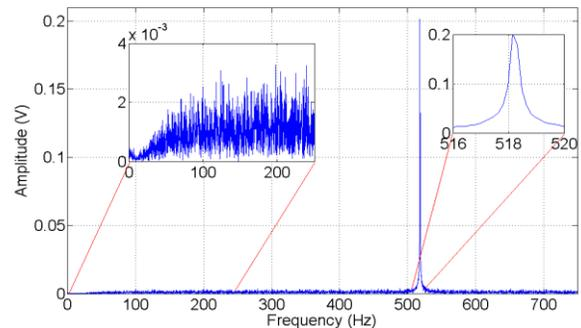
Fig. 7. The spectrum of AM-demodulated recorded signal in impulse interrogation approach.
