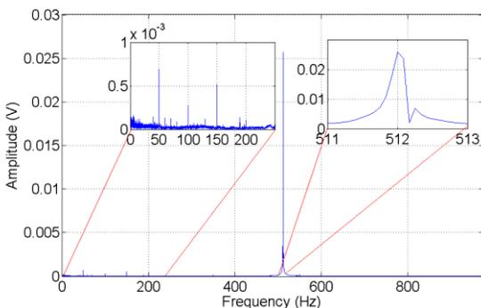
Fig. 5 The spectrum of FM-demodulated recorded signal of the oscillator with rotation.
