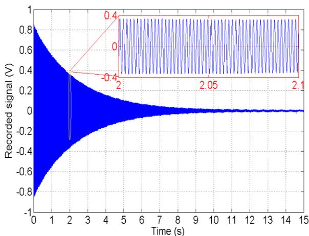
Fig. 3. Recorded FM-demodulated signal of the oscillator with a SAW resonator under fast varying deformation.
