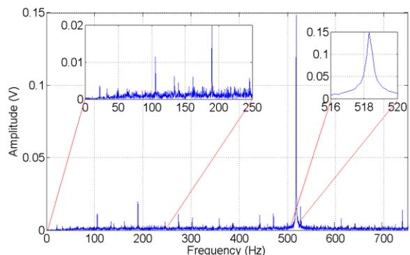
Fig. 8. The spectrum of AM-demodulated recorded signal in impulse interrogation approach with rotation.
