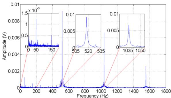
Fig. 11. The spectrum of FM-demodulated recorded signal with rotation.
