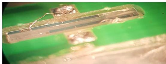
Fig. 1. Wire bonding connection of the sensor PC-board and SAW-resonator sensor interdigital transducer with a gold conductor.
