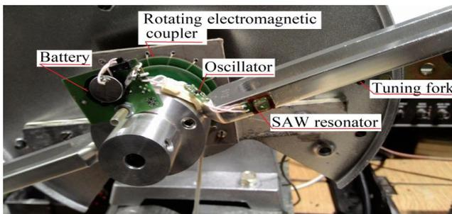
Fig. 2. Vibration sensor test setup including: rotating electromagnetic coupler, tuning fork, SAW resonator, oscillator and battery.
