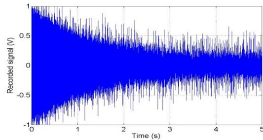
Fig. 6. Recorded vibration related signal after AM-demodulation without rotation.
