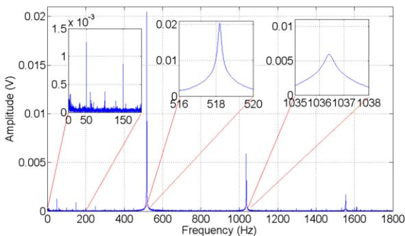
Fig. 10. The spectrum of FM-demodulated recorded signal.
