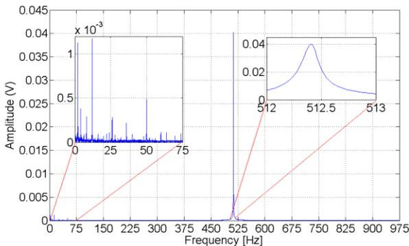
Fig. 4. The spectrum of FM-demodulated recorded signal of the oscillator without rotation.
