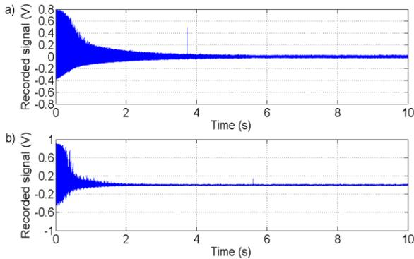
Fig. 9. Recorded signal after FM-demodulation of: a) the signal related to vibration without rotation, b) the signal related to vibration with rotation of the vibrating object.
