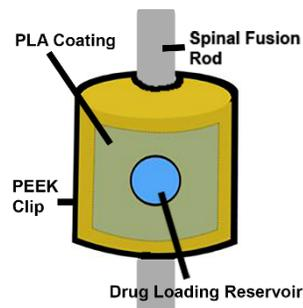
Fig. 1. Representative image of 1-hole PEEK clip for US-triggered drug delivery (not to scale).
