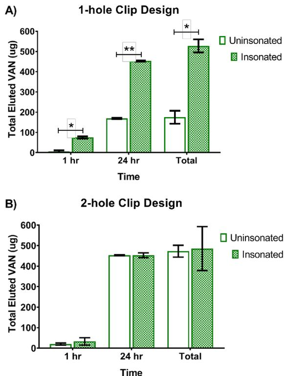
Fig. 2. *In vitro* characterization of VAN release from 1-hole and 2-hole PEEK clip designs, represented as average  $\pm$  SD. A) Elution of VAN from the 1-hole clip, \*p = 0.0002, \*\*p < 0.0001. B) Elution of VAN from the 2-hole clip.
