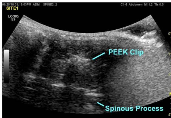
Fig. 3. Representative US image of PEEK clip implanted in the *ex vivo* rabbit spine model.
