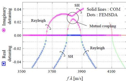
Fig. 3. Dispersion characteristics calculated by FEM/SDA<sup>[13][14]</sup> and proposed multi-mode COM model.
