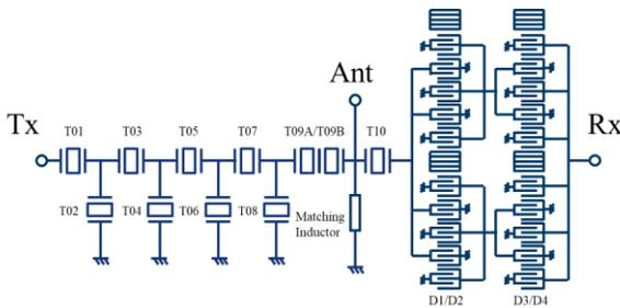
Fig. 9. Circuit topology of LTE Band8 duplexer.
