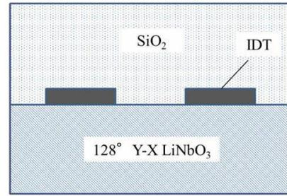
Fig. 1. Cross sectional view of TC-SAW structure.
