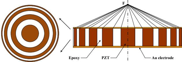
Fig. 1. Schematic of Micromachined Self-focusing Piezoelectric Composite Ultrasound Transducer
