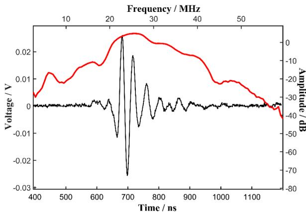
Fig. 5 The pulse-echo waveform and frequency spectrum of fabricated FPCUT transducer
