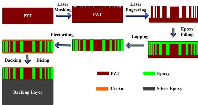
Fig. 3 Schematic process flow for micromachined self-focusing piezoelectric composite
