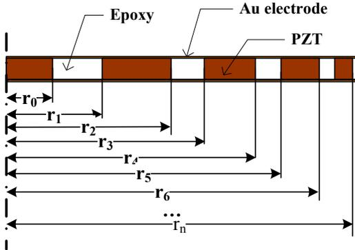
Fig. 2. The annular rings in PZT to focus the acoustic waves.
