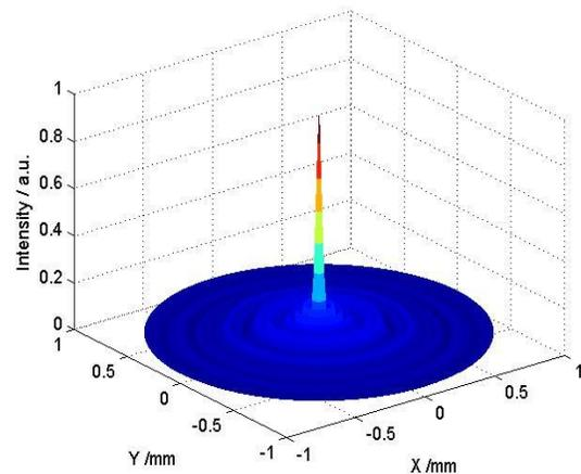
Fig. 7 Measured acoustic intensity distribution of fabricated FPCUT
