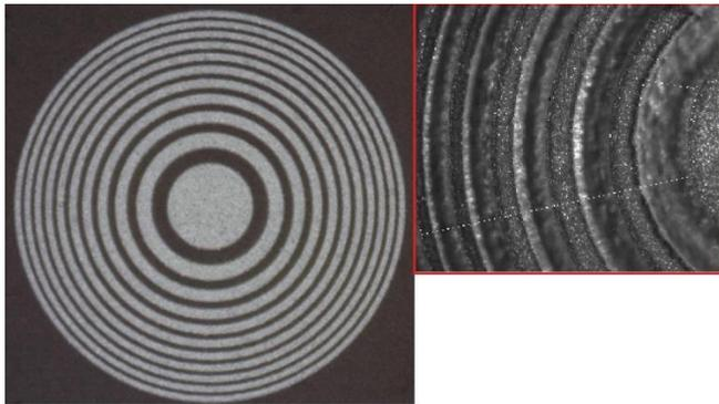
Fig. 4 Photographs of the engraved Fresnel annulus piezocomposite
