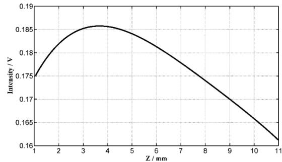
Fig. 6 The measurement acoustic intensity of fabricated FPCUT along Z axis
