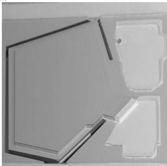
Fig.2; Cantilever type ZDR. The resonator is held at only one point (right side). This attachment point also is used for the electrical contacts to the resonator.
