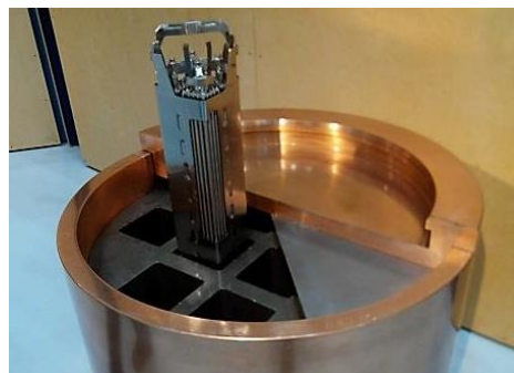
Fig. 1. Partial section of a copper canister with iron insert hosting a spent fuel assembly.
