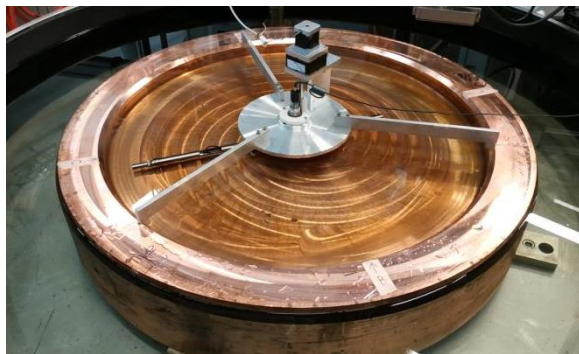
Fig. 4. New version of the ultrasonic reader prototype during test on a real copper lid already welded onto the canister.
