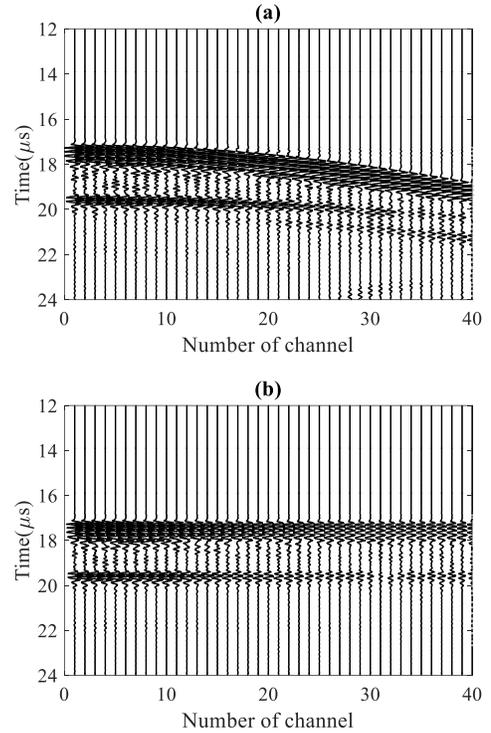
Fig. 3 The received signals of the first 40 channels, (a) the origin signals; (b) the CS adjusted signals.
