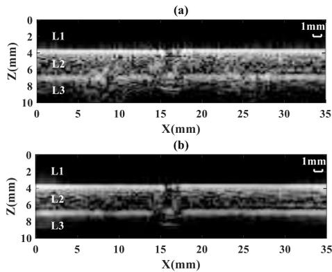
Fig. 4 Experiment results, (a) reconstructed image using SAFT; (b) reconstructed image using MSAU. L1, L2, and L3 indicate the three layers, water, cortical bone, water, respectively.
