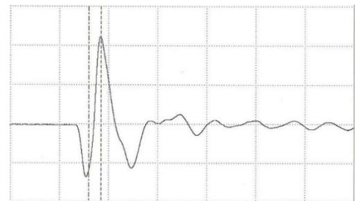
Fig. 8 Pulse response (500 nsec/div, 100 mV/div) of type 855 piezoelectric wafer prepared using the vacuum assisted slip casting process with pore density  $1050 \text{ mm}^{-2}$ , diced at  $750 \mu\text{m}$  pitch.
