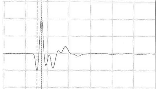
Fig. 6 Pulse response (500 nsec/div, 100 mV/div) of manufacturer-supplied APC type 855 piezoelectric wafer diced at  $750 \mu\text{m}$  pitch, with factor of 4 sub-dicing. Note the much cleaner response following the leading edge of the pulse compared to Fig. 5 without sub-dicing.
