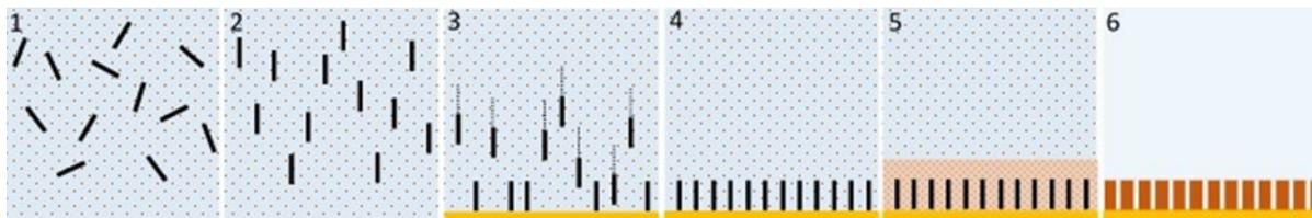
Fig. 1 Process for producing oriented pore ceramic material by magnetic alignment of nickel-coated fibres as described in the text
