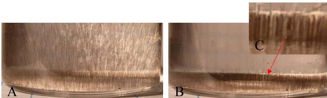
Fig. 2. Fibres in PZT slurry mimicking solution, A. 2 sec post filling container, B. at 20 sec, C. magnified image of area indicated.
