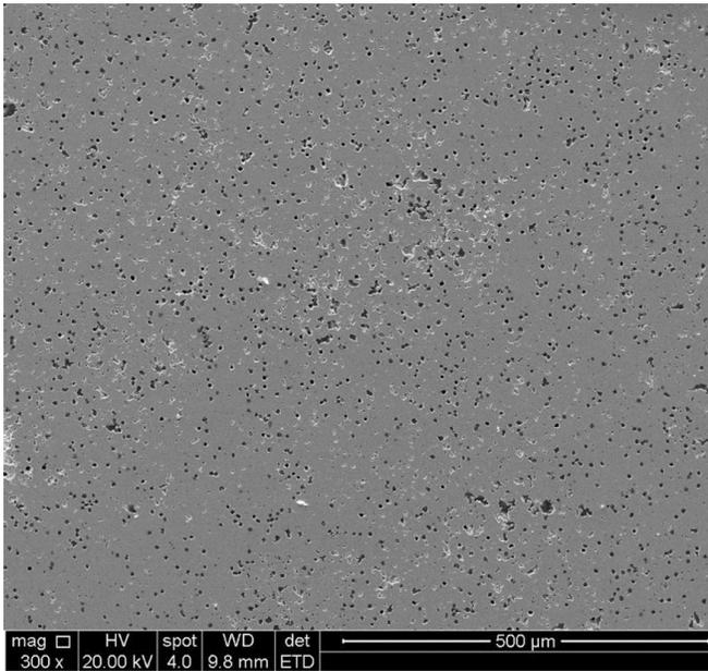
Fig. 3 SEM image of a section of a sintered wafer
