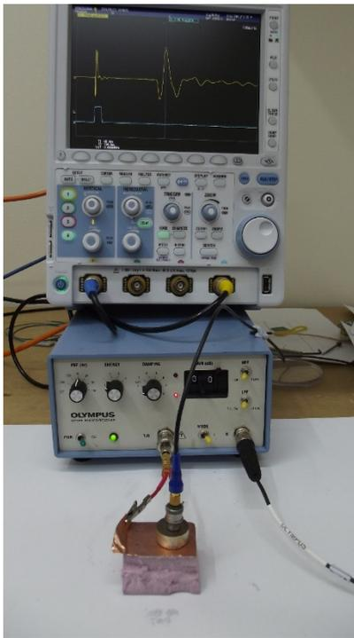
Fig. 4 Ultrasonic measurement setup
