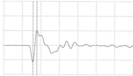
Fig. 5 Pulse response (500 nsec/div, 100 mV/div) of manufacturer-supplied APC type 855 piezoelectric wafer diced at  $750 \mu\text{m}$  pitch. This material was prepared by a standard pressing and sintering process.
