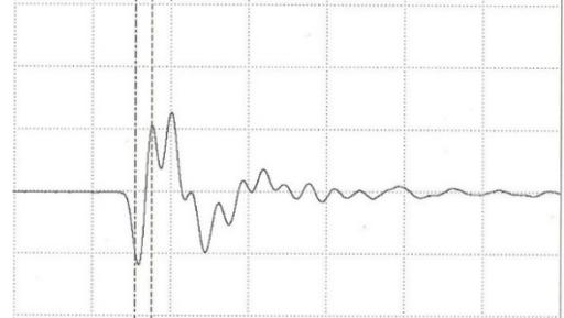
Fig. 7 Pulse response (500 nsec/div, 100 mV/div) of type 855 piezoelectric wafer prepared by using the vacuum-assisted slip casting procedure with a low pore density  $50 \text{ mm}^{-2}$ , diced at  $750 \mu\text{m}$  pitch.
