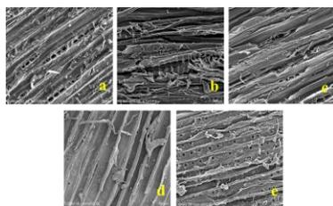
Fig. 2. SEM images of biochar derived from ultrasound pre-treated wood chips. a) Untreated b) UST 1 c) UST 2 d) UST 3 e) UST 4
