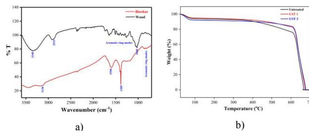
Fig. 1. a) Infrared spectra of feedstock and biochar derived. b) Thermogravimetric analysis of ultrasound untreated and pre-treated wood biochar
