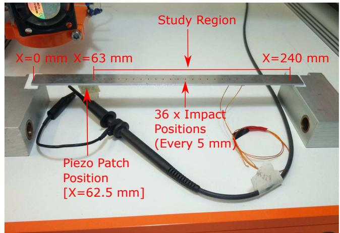
Fig. 2. An aluminum beam is mounted on the Stepcraft 600 CNC table using double sided tape. A piezoelectric patch is stuck under the beam at position  $x = 62.5$  mm, and the study region goes from  $x = 63$  mm and goes until 240 mm
