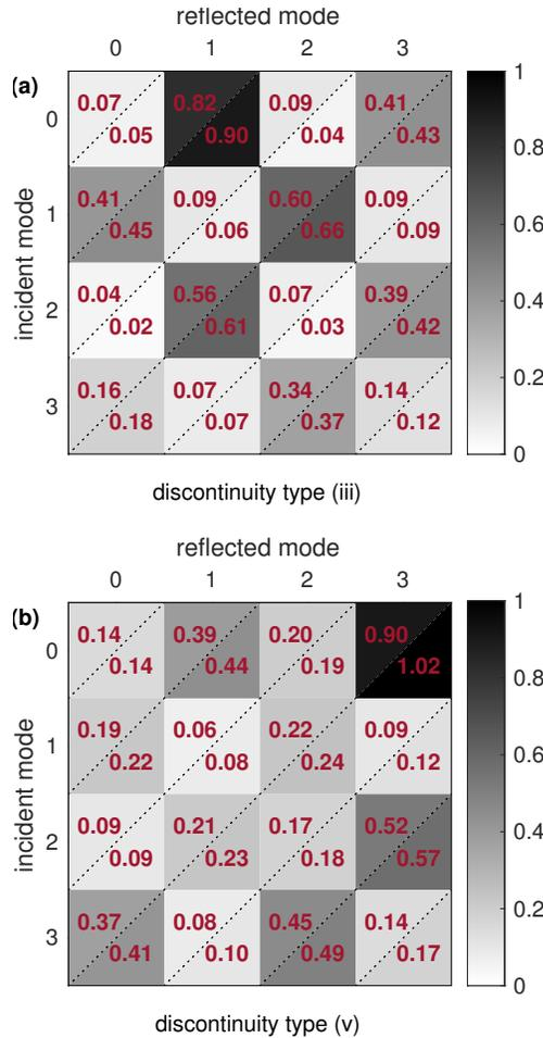
Fig. 4. Reflection coefficients due to the interaction of SH guided wave modes with discontinuities types (iii) and (v). The colormap represents the intensity of the reflection coefficient. Upper triangles represent the case in which the fixed half of the discontinuity is simulated with a filling material whose impedance is  $Z_d = 10 \times Z$ , whereas lower triangles when using fixed boundary conditions.
