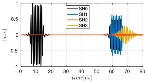
Fig. 2. Interaction of the SH0 mode with a half-thickness non-symmetric discontinuity. Incident mode, at  $\sim 10\mu s$ , and reflected modes at  $\sim 60\mu s$ .
