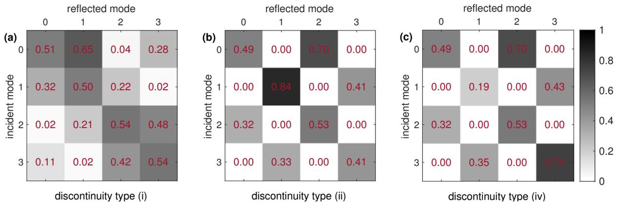
Fig. 3. Reflection coefficients due to the interaction of SH guided wave modes with discontinuities types (i) (ii) and (iv). The colormap represents the intensity of the reflection coefficient. The numerical values of the reflection coefficients are shown in each cell.
