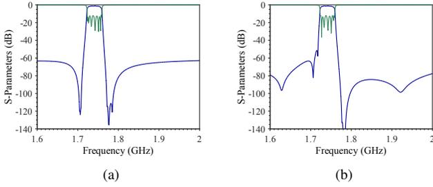
Fig. 2. S-parameters of a (a) plain ladder filter and the same filter with a GLI (b) between resonators 2 and 4.
