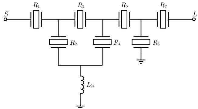
Fig. 1. Example of 7th-order filter with GLI cross-coupled inductor between resonators 2 and 4.
