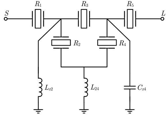
Fig. 3. Scheme of the 5th-order filter with a GLI in resonators 2 and 4.
