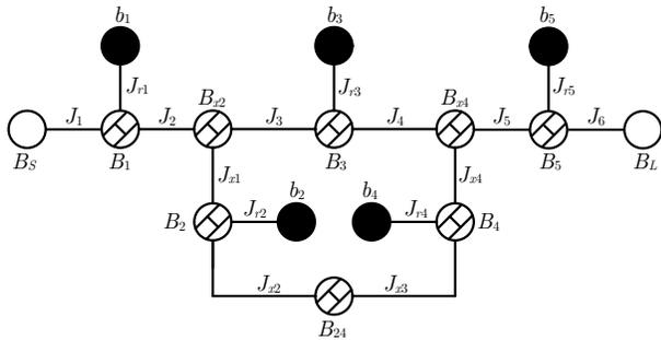
Fig. 6. Scheme of the 5th-order filter with a GLI in resonators 2 and 4.
