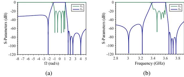
Fig. 7. S-parameters of (a) the lowpass response of the 5th-order filter and (b) the bandpass response.
