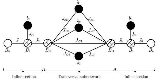
Fig. 4. Lowpass prototype nodal scheme of a 5th-order mixed-topology fully canonical filter.
