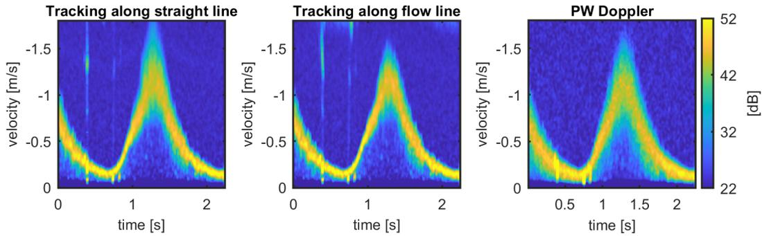
Figure 3. Tracking Doppler and PW Doppler spectra generated from the recorded flow phantom shown in Figure 4. The tracking Doppler spectra were estimated along the 2 cm long straight and curved trajectories shown in the picture. The PW Doppler sample volume was placed at the middle of the tracking trajectories.
