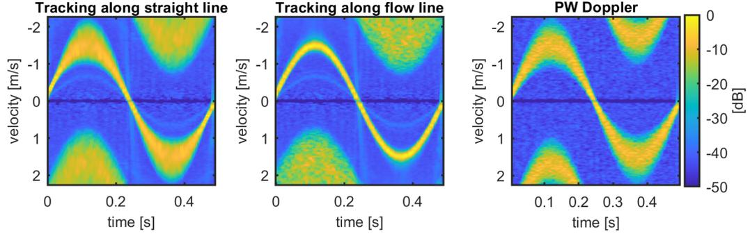
Figure 1. Tracking Doppler and PW Doppler spectra generated from the simulated flow phantom shown in Figure 2. The tracking Doppler spectra were estimated along the 2 cm long straight and curved trajectories shown in the picture. The PW Doppler sample volume was placed at the middle of the tracking trajectories.
