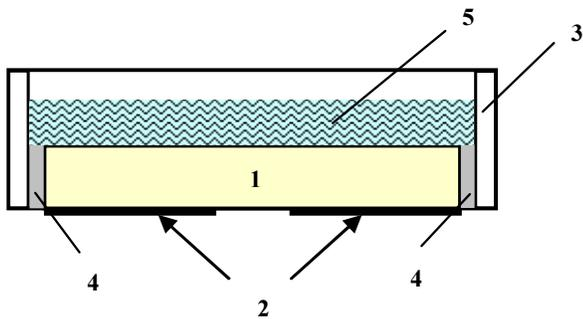
Fig. 1. The scheme of the sensor: 1 – the plate of the PZT ceramics, 2 – electrodes, 3 – the liquid container, 4 – the adhesive sealant, 5 – cell suspension under study.
