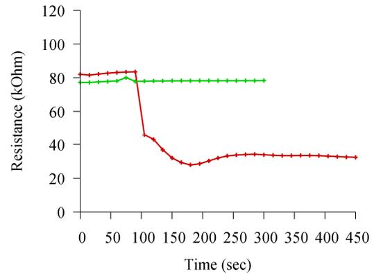
Fig. 4. The time dependences of the maximum of real part of the electrical impedance of PZT resonator during a specific interaction “*A. brasilense* Sp7 cells – specific antibodies” (red line) and nonspecific interaction “*E. coli* XL-1 cells – non-specific antibodies” (green line) for the resonance peak near 68.7 kHz.
