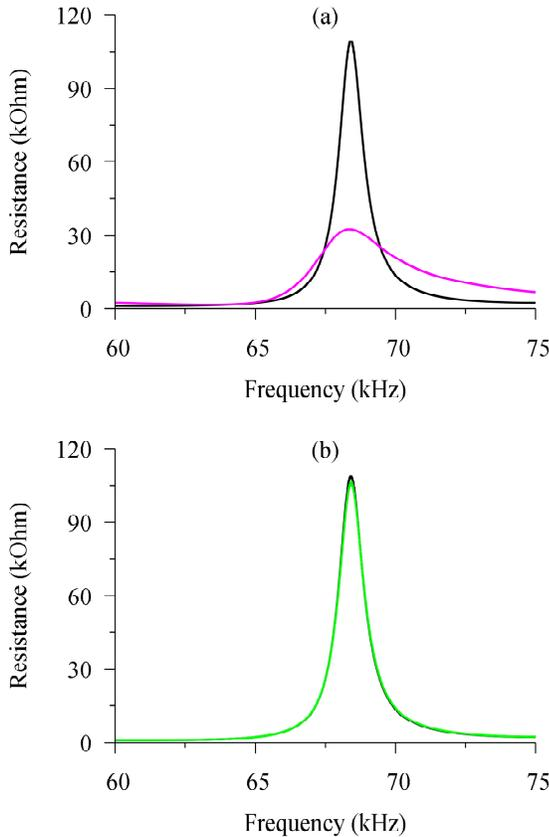
Fig. 3. The frequency dependencies of the real part of the electrical impedance of PZT resonator: (a) – container with *A. brasilense* Sp7 cells before (black curve) and after (pink curve) adding the specific antibodies; (b) – container with *E. coli* XL-1 cells before (black curve) and after (green curve) adding the non-specific antibodies.
