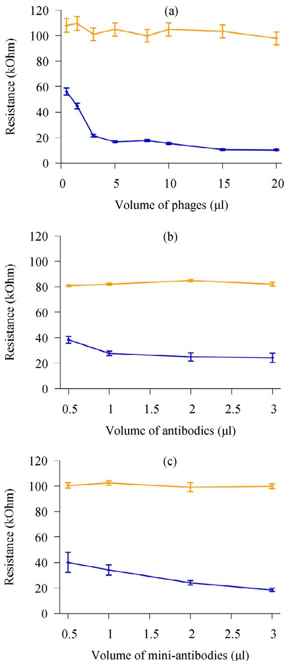
Fig. 5. Dependences of the maximum value of real part of electrical impedance of the resonator on the number of specific reagents added to microbial cells: (a) – E. coli XL-1 + phage M13K07; (b) – A. brasilense Sp7 + antibodies; (c) – A. brasilense Sp245 + mini-antibodies.
