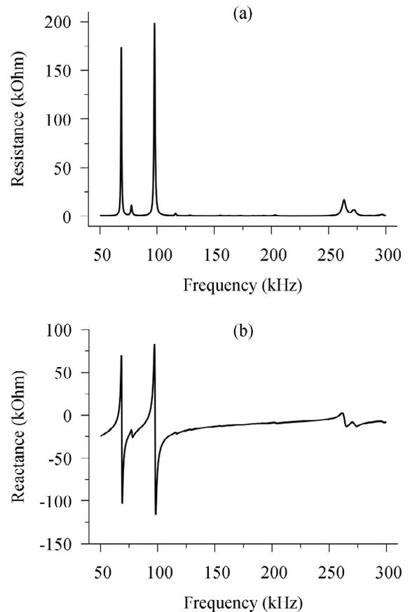
Fig. 2. The frequency dependences of the real (a) and imaginary (b) parts of the electrical impedance of PZT resonator with empty liquid container.
