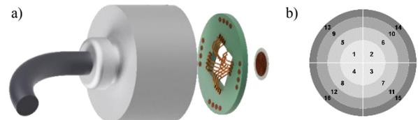
Fig. 3: a) Schematic drawing of the probe: (from left to right) connecting cables, housing with damping body, interconnection layer, transducer with electrodes structured as annular-array; b) structure of the annular-array.
