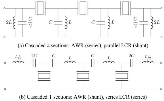
Fig. 4. Cascaded filter stages ( $N = 3$ )
