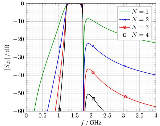
Fig. 5. Filter transmission (calculation) of  $N$  cascaded  $\pi$ -type example filter stages ( $N = 1$  to 4)
