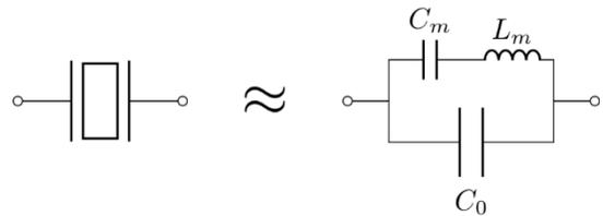
Fig. 1. Lossless BVD model of an acoustic-wave resonator
