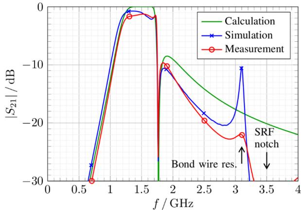
Fig. 7. Filter transmission of a single example filter stage: Comparison of calculation with ideal elements (green), simulation including PCB effects, bond wires, and S-parameter models of elements (blue), and measurement of discrete structure (red)
