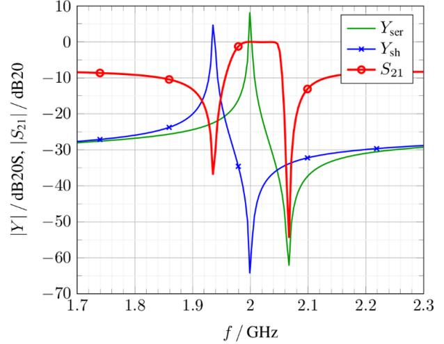
(b) Resonator admittance and filter response
