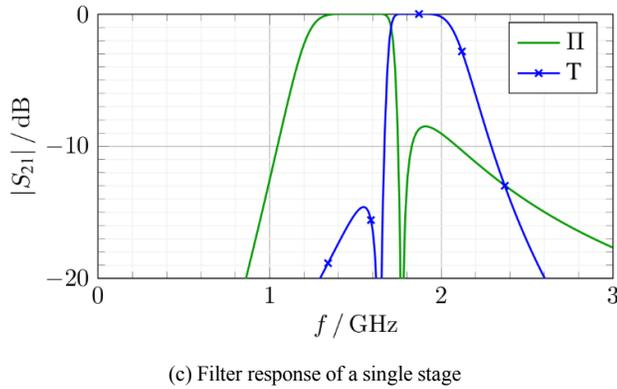
Fig. 3. Working principle of the two presented complementary filter stages
