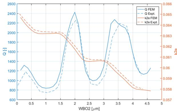
Fig. 3: Quality factor,  $Q$ , and effective coupling,  $k_{2e}$ , calculated with the 2D FEM model as a function of the width of the raised frame,  $WBO_2$ , and compared to experimental data from a regular 3D device.
