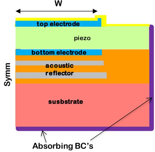
Fig. 2: Energy leakage and boundary conditions (BC's) for a SMR with raised frame or border ring. The absorbing BC's should prevent the reflections of acoustic waves at the truncations of the system.
