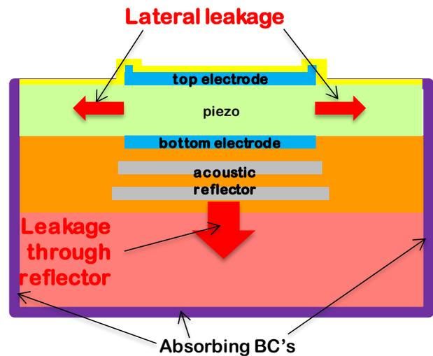
Fig. 1: Typical cross-section of a Solidly Mounted Resonator consisting of a piezoelectric layer, top and bottom electrodes, and an acoustic mirror. Energy leakage and boundary conditions (BC's): the absorbing BC's should prevent the reflections of acoustic waves at the truncations of the system.
