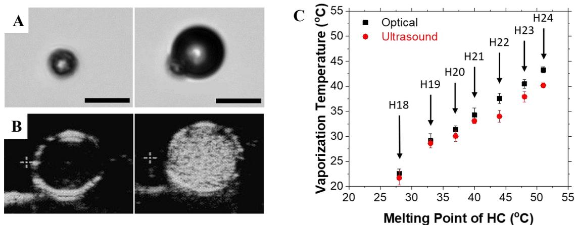
**Figure 1** | **A** Optical microscopic image of a droplet before and after vaporization. Scale bar 20  $\mu\text{m}$ . **B** Contrast-enhanced ultrasound image of the droplet solution inside dialysis tubing before vaporization and after vaporization of the droplets. **C** Linear correlation of the vaporization temperature of endoskeletal droplets and the melting point of the solid hydrocarbon.
