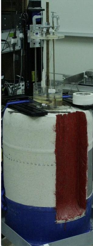
Fig 5. Simulated borehole with Plexiglas casing to mimic the open borehole configuration
