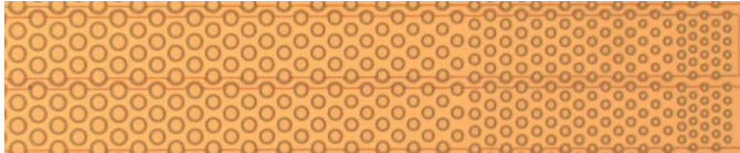
Fig. 1. Optical image of PMUT cell arrangement in an element. A section of the transducer element shown in picture.
