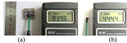
Fig.4. (a) The fabricated planar magnet array. (b) A single permanent magnet.
