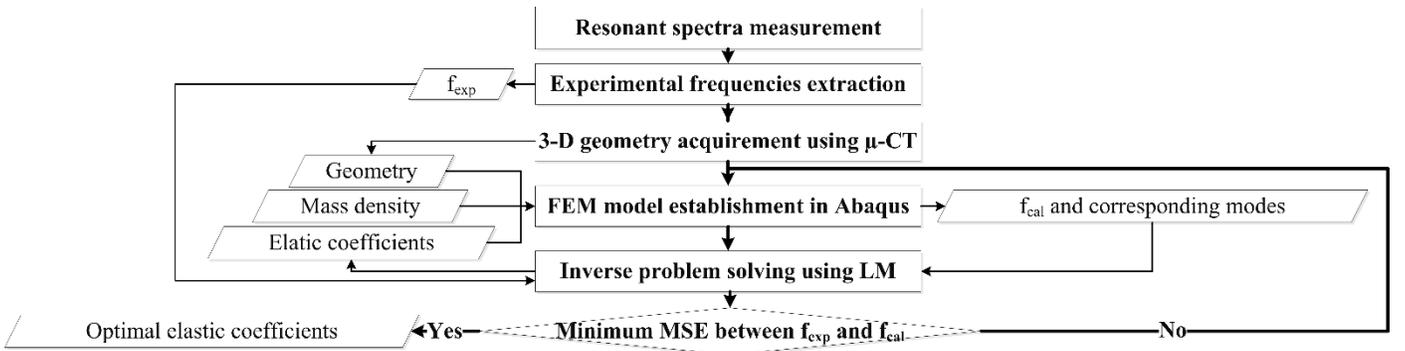
Fig. 1. The flowchart of RUS combined with FEM and  $\mu$ -CT.
