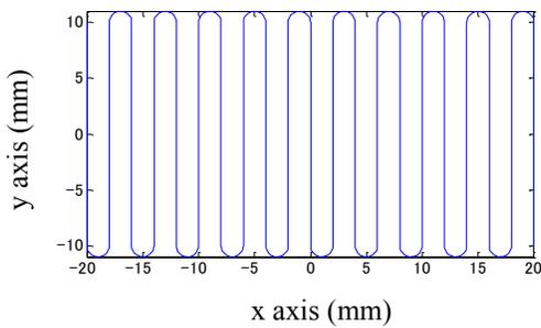
Fig. 2 Motion of the hemispherical sensor array during 2D scanning
