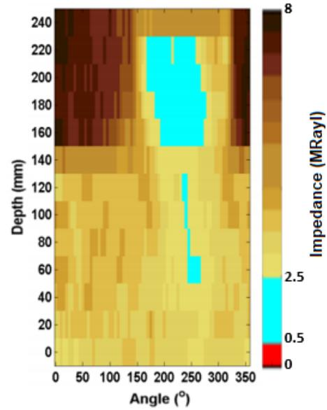
Fig. 5. Pulse-echo impedance map of cemented sample.
