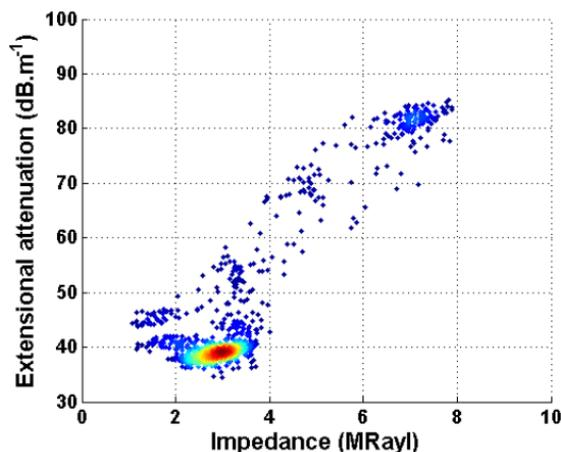
Fig. 7. Cross-plot of extensional attenuation versus pulse-echo impedance.
