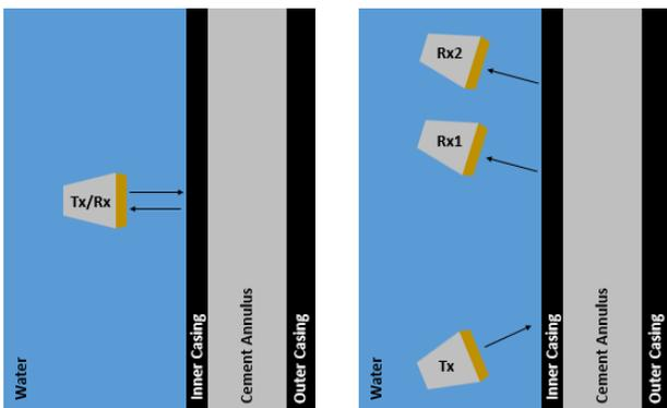
Fig. 4. (Left) Pulse-echo thickness mode and right Pitch-catch extensional mode measurement setup.
