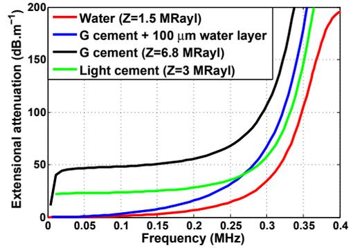
Fig. 3. Modal attenuation of the zero order symmetrical mode of a 6.5 mm thick steel plate using Disperse [16] for various materials adjacent to it.
