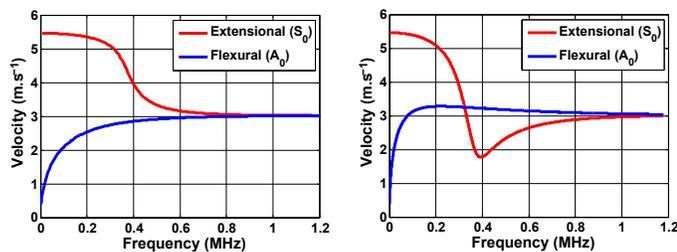
Fig. 2. Phase velocity (left) and group velocity (right) in vacuum in a 6.5 mm steel plate. (from Disperse [16])
