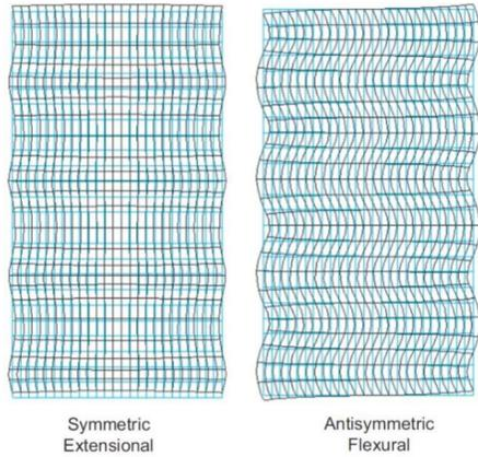
Fig. 1. Representation of the motion of the both zero-order symmetrical and anti-symmetrical mode of a guided wave in a steel plate. (from Disperse [16])
