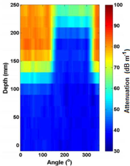
Fig. 6. Extensional attenuation map of cemented sample.
