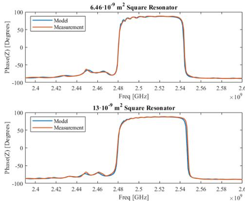
Fig. 6. Phase of the input impedance of the two square resonators.
