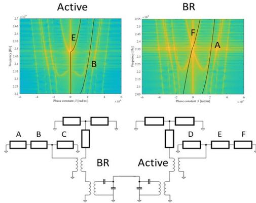
Fig. 4. Circuitual model for the BR modes. The dispersion curves correspondents to each lateral transmission line section are shown on top. C and D are lumped resistances.
