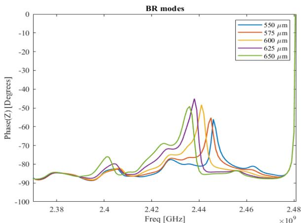
Fig. 2. Different BR modes depending of the BR width (from 5.5  $\mu\text{m}$  to 6.5  $\mu\text{m}$ ).
