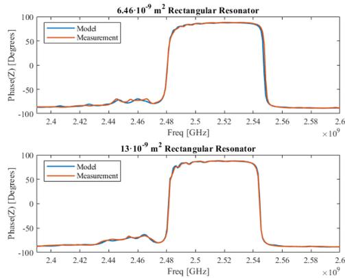
Fig. 7. Phase of the input impedance of the two rectangular resonators
