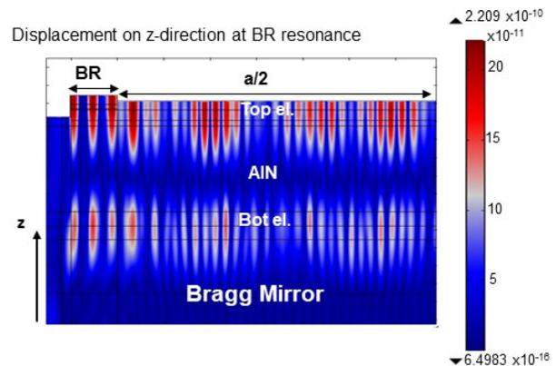
Fig. 3. FEM simulation of a SMR. The displacement field on the thickness direction is shown.
