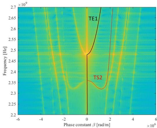
Fig. 1. Dispersion curves of an AlN piezolayer SMR. The fundamental mode TE<sub>1</sub> is fitted to the black curve and the TS<sub>2</sub> to the red one. Type I dispersion behavior can be seen.
