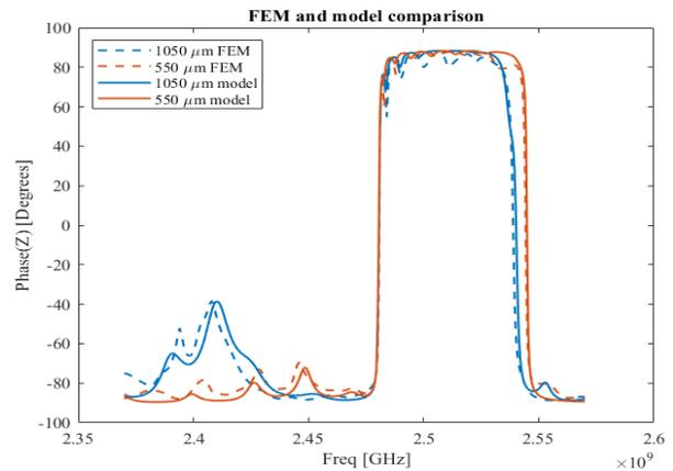
Fig. 5. Phase of the input impedance of FEM simulated SMR (dotted traces), and adjustment of our model (solid traces). Blue traces correspond to a BR width of 5.5  $\mu\text{m}$ , while red to 10.5  $\mu\text{m}$ .
