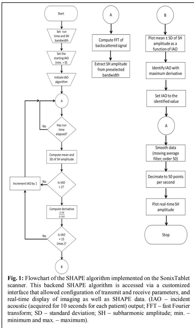
**Fig. 1:** Flowchart of the SHAPE algorithm implemented on the SonixTablet scanner. This backend SHAPE algorithm is accessed via a customized interface that allowed configuration of transmit and receive parameters, and real-time display of imaging as well as SHAPE data. (IAO – incident acoustic (acquired for 10 seconds for each patient) output; FFT – fast Fourier transform; SD – standard deviation; SH – subharmonic amplitude; min. – minimum and max. – maximum).
