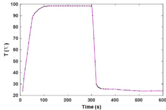
(b) The heating and cooling curve of the micro-heater
