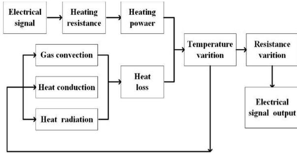
Fig.2 The working principle of micro-heater
