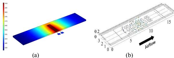
Fig. 4 COMSOL simulation:(a)Temperature distribution of Micro-heater (b)The thermo-deposition distribution of particles when the micro-heater is located above the intermediate IDT.
