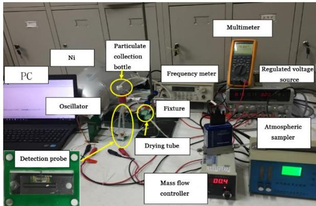
Fig.7 The experimental system
