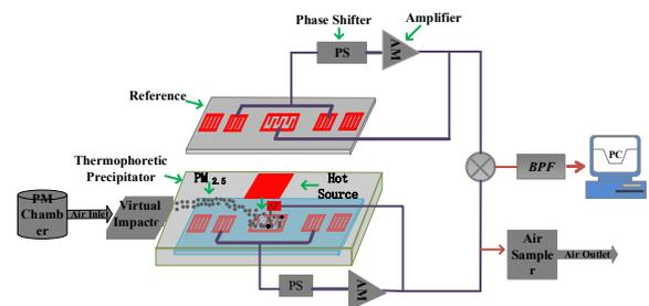
Fig.1 The schematic of the novel SAW-based PM<sub>2.5</sub> monitor.
