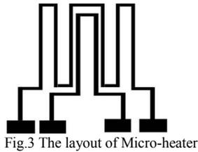
Fig.3 The layout of Micro-heater
