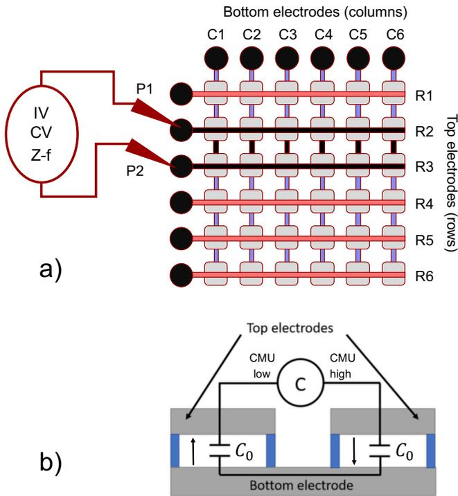
Fig. 2. a) Illustration of the measurement of the capacitance between two neighboring top electrodes,  $R2$  and  $R3$  using two probes,  $P1$  and  $P2$ . b) The bottom electrodes,  $C1$  to  $C6$ , effectively connect the CMUT cell capacitors in  $R2$  in series with the cell capacitors in  $R3$ . The measured capacitance is therefore  $C = C_0/2$ . The arrows show the direction of the electric field in the CMUT cavities. The electric field points in opposite directions.
