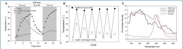
Fig. 1. The photothermal conversion performance of AuNR and ICG in various experimental parameters. A. Experimental temperature traces of AuNR, ICG and PBS under CW laser irradiation. B. The influence of CTAB concentration on the photothermal conversion performance of AuNR. C. The photoacoustic signal of AuNR and ICG in different solutions under pulsed laser irradiation.
