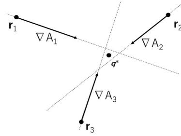
Fig. 2. Lines parallel to the gradient ideally converges at the microphone location.
