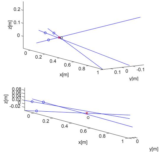
Fig. 5. Localization results and gradient lines for microphone located at  $(160, 0, 10)$  [mm] (Upper Figure) and at  $(535, 0, 10)$  [mm] (Lower Figure). Blue circles, black circles and red stars indicate the source positions, the true microphone positions, and the estimated microphone positions.
