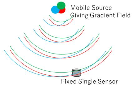
Fig. 1. Our strategy to achieve single microphone localization based on sources with small tunable displacement.
