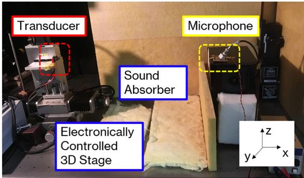
Fig. 4. Experimental setup.
