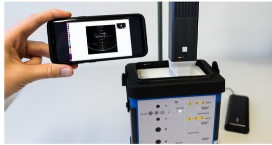
Fig. 5. Our wireless probe and a smartphone displaying in real-time the forwarded SASB image computed on a PC connected to the same network. The probe is powered over USB with a battery pack visible in the background.
