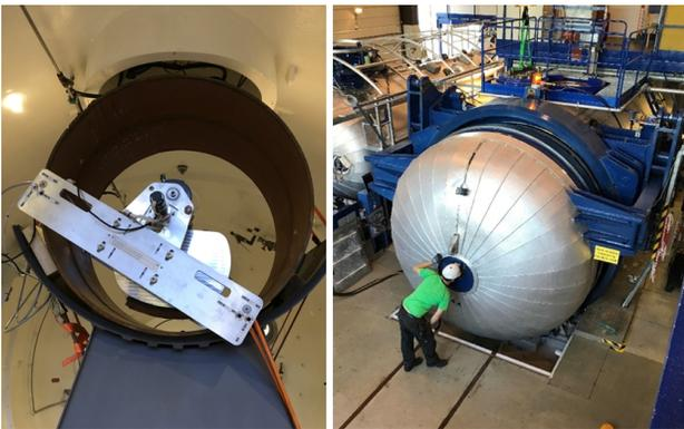
Fig. 3. Picture of the set-up inside the pressure chamber (left) and of the pressure chamber at the Norwegian Underwater Institute (right).
