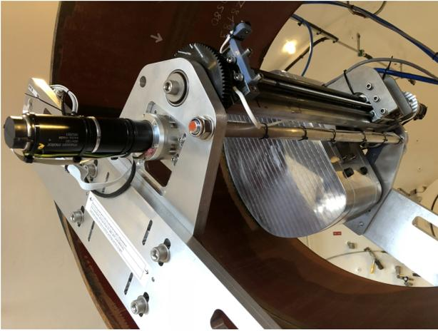
Fig. 2. Set-up of the test scanner inside a pipe sample.
