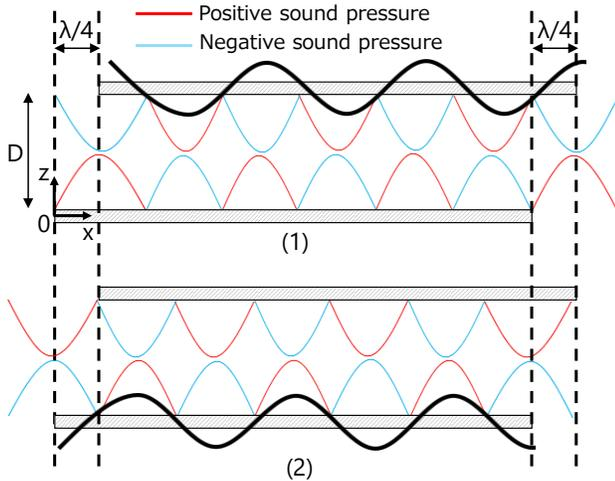
Fig. 2. Sound pressure distribution when only one side vibration plate is driven: (1), upper; (2), lower.
