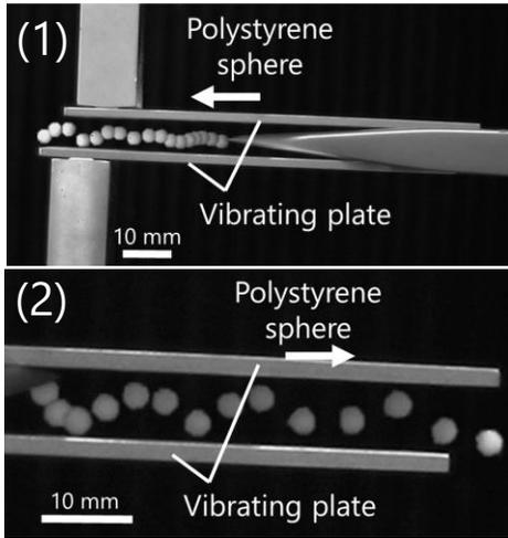
Fig. 6 Photo of the transportation trajectory of a polystyrene sphere between the vibrating plates taken at every 10 ms: (1), left direction; (2), right direction.
