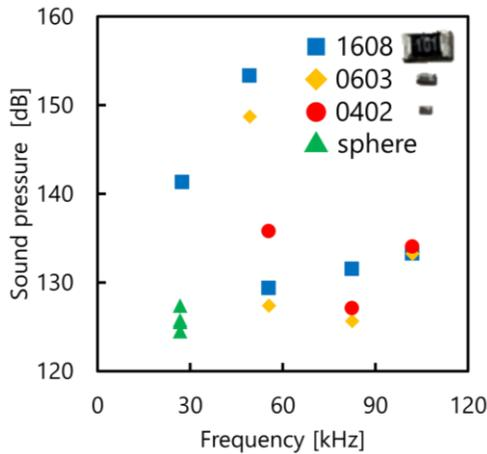
Fig. 12 Relationship between frequency and size of levitating objects.
