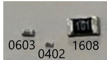
Fig. 10 Photo of the chip parts.
