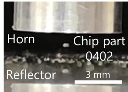
Fig. 11 Photograph of levitating a chip part 0402.
