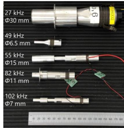
Fig. 9 Transducers used in the experiment.
