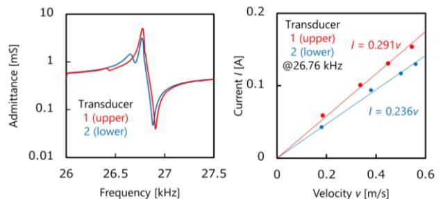
Fig. 5. Admittance characteristics (left) and force factors of transducers measured at 26.76 kHz (right).
