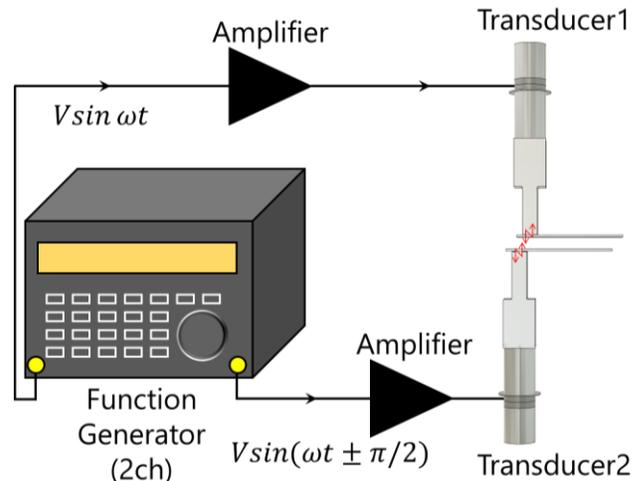
Fig. 3. Excitation method of two transducers with phase difference.
