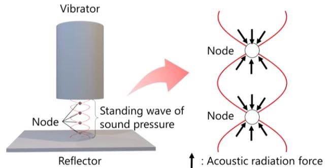
Fig. 1. Principle of ultrasonic levitation.
