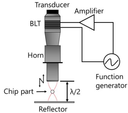
Fig. 8 Experimental setup for levitation of chip parts.
